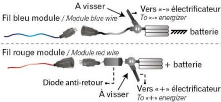
Fig. 50 - Branchement ABS / Connecting ABS
